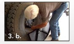
**3. b.** Install socket on the lug nut, slide **Torque Fin**<sup>®</sup> on the extension until it touches side wall of the tire.
