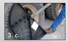
**3. c.** Use your foot to press **Torque Fin**<sup>®</sup> against the ground.
