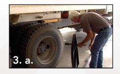
Torque lug nuts with torque wrench and Torque Fin<sup>®</sup>.
