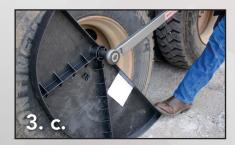
**3. c.** Use your foot to press **Torque Fin**<sup>®</sup> against the ground.
