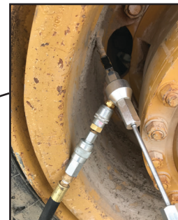
D. Large Bore Core Tool fastens to the valve for faster flow during inflation/deflation.
