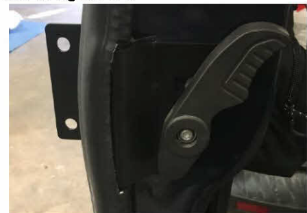
Figure 12: Installed Weather Stripping After Modification
