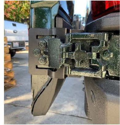
Figure 5: Inside View of Installed Lower Hinge Bracket
