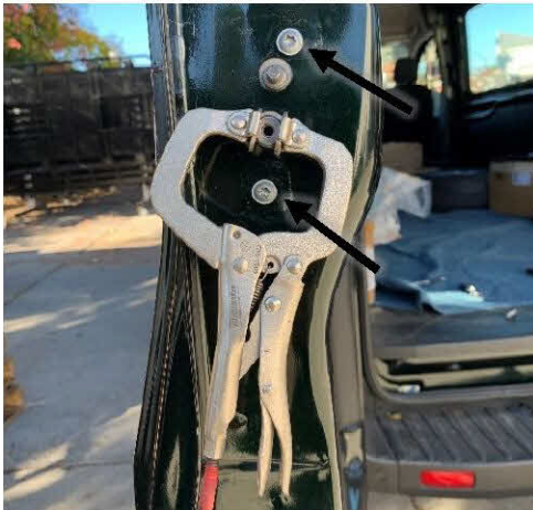
Figure 8: Inner Driver Door Bracket Installed
