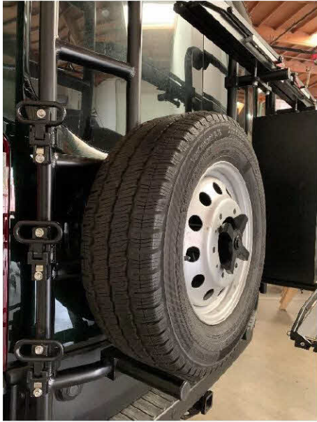
Figure 5: Tire Mount Assembled
