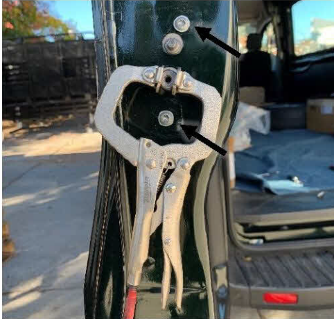
Figure 7: Inner Door Bracket Installed
