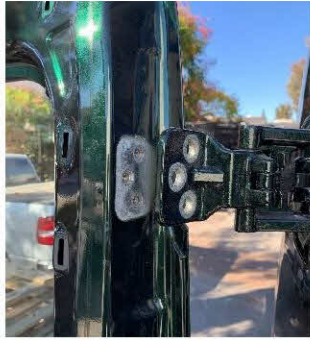
Figure 2: Upper Hinge Rotated Away from Door
