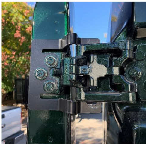
Figure 4: Inside View of Installed Upper Hinge Bracket
