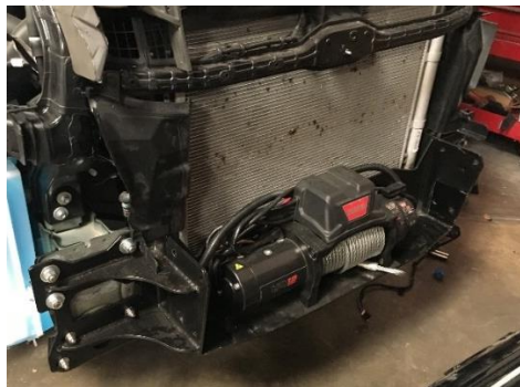
Figure 29: Winch Installed onto Winch Plate
