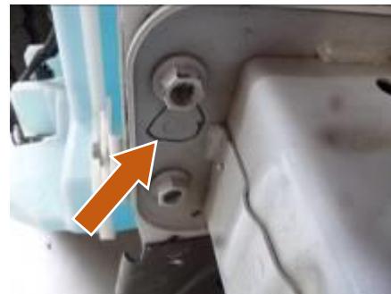
Figure 22: Example of Spot Weld (Shown from the Back)
