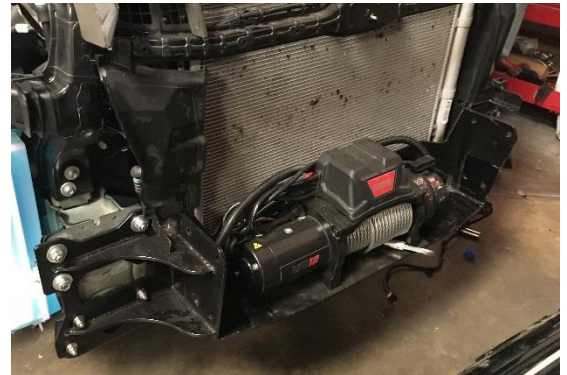
Figure 30: Winch Installed onto Winch Plate
