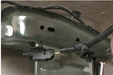
Figure 18: Temperature Sensor Removed
