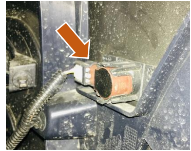
Figure 15: Parking Sensors from Backside of Bumper
