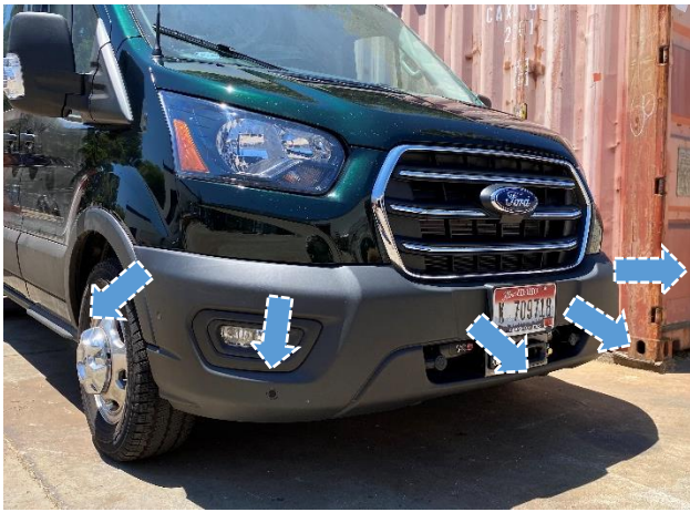
Figure 12: Factory Bumper Removal
