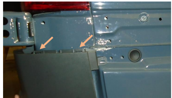
Figure 8: Small Plastic Panel Removed
