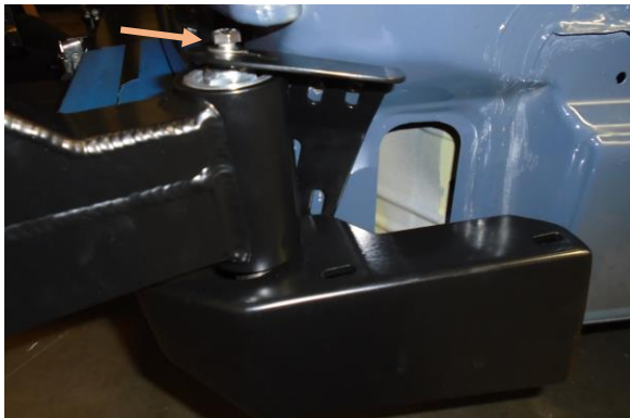
Figure 10: Pre-Mounting Axle Support Brackets
