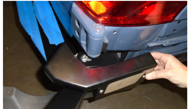
Figure 13: Installation of the Trim Assembly
