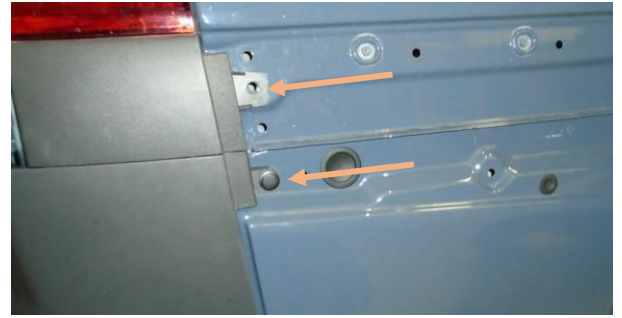
Figure 6: Plastic Rivets Underneath the Side Panel
