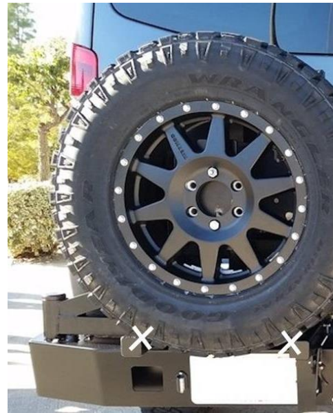
Figure 15: Tire Resting Correctly on Swing Arm
