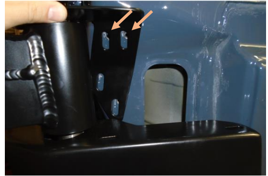
Figure 11: Drilling for Axle Support Bracket
