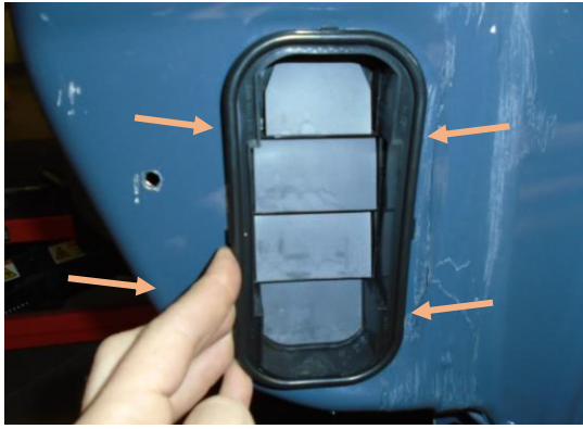
Figure 9: Air Pressure Relief Insert Removal
