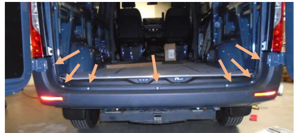
Figure 2: Torx Bolts on the Rear Bumper
