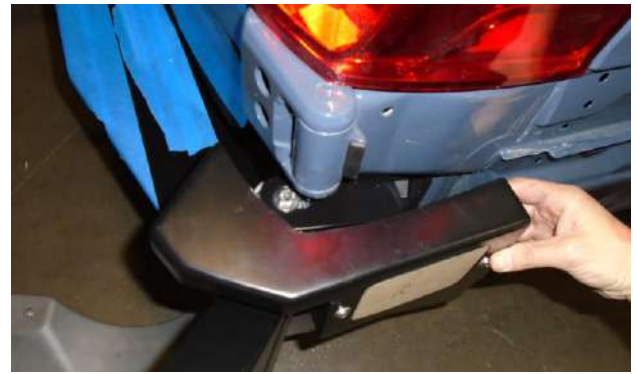
Figure 13: Installation of the Trim Assembly
