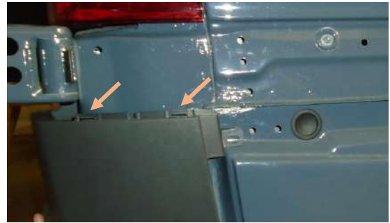
Figure 8: Small Plastic Panel Removed
