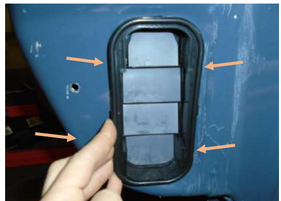
Figure 9: Air Pressure Relief Insert Removal
