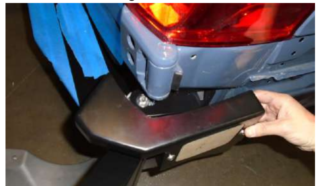
Figure 13: Installation of the Trim Assembly
