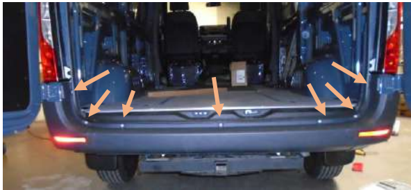
Figure 2: Torx Bolts on the Rear Bumper
