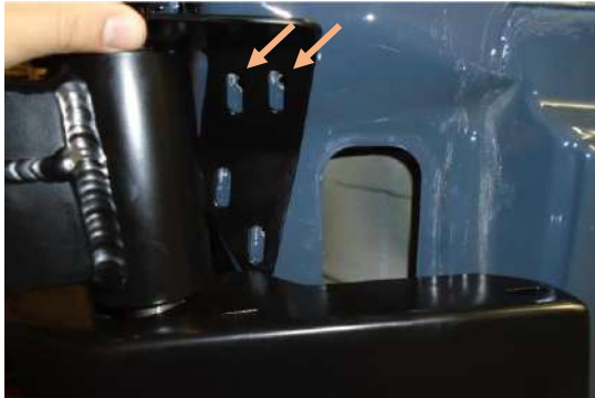
Figure 11: Drilling for Axle Support Bracket
