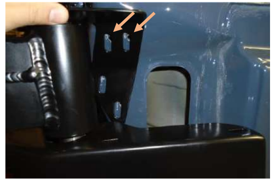
Figure 11: Drilling for Axle Support Bracket
