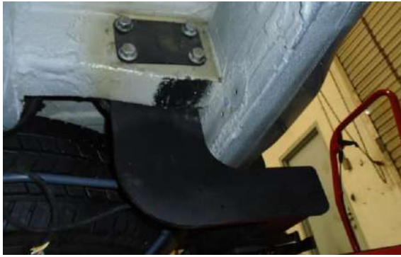
Figure 1: Four (4) of the Hitch Mounting Bolts
