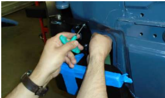
Figure 12: Tightening Hardware Through Insert Opening
