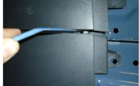
Figure 7: Removing Small Plastic Panel from Rear Bumper
