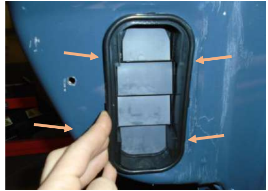
Figure 9: Air Pressure Relief Insert Removal
