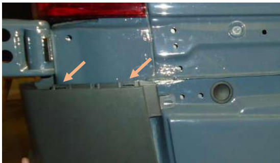
Figure 8: Small Plastic Panel Removed
