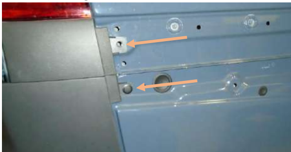
Figure 6: Plastic Rivets Underneath the Side Panel
