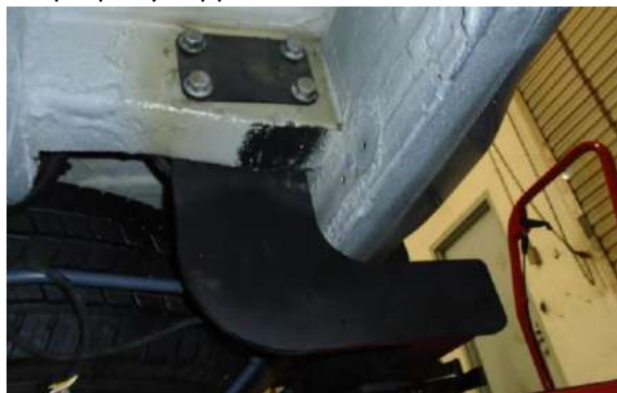
Figure 1: Four (4) of the Hitch Mounting Bolts
