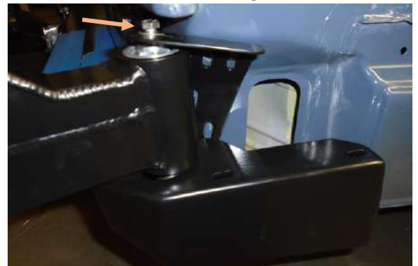
Figure 10: Pre-Mounting Axle Support Brackets
