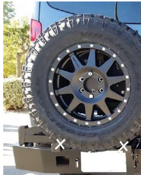
Figure 16: Tire Resting Correctly on Swing Arm
