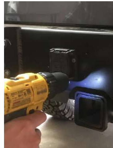
Figure 15: Installation of the trailer plug
