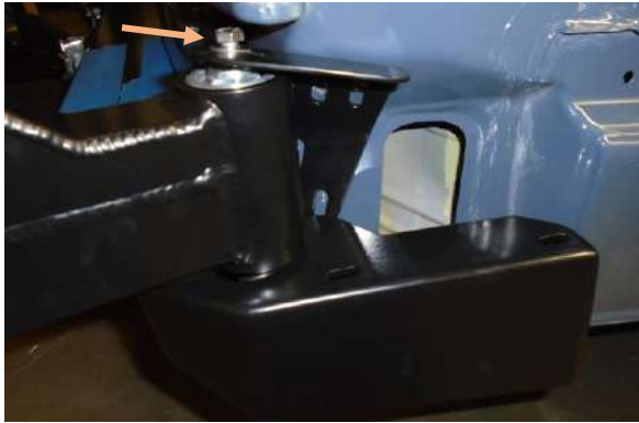
Figure 10: Pre-Mounting Axle Support Brackets
