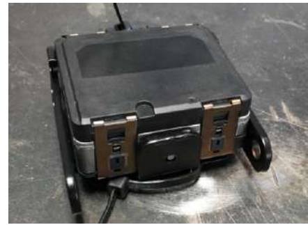
Figure 25: Tighten Zip Tie(s) Around Top of Sensor Carriage
