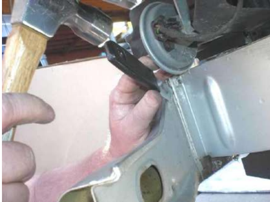
Figure 13: Releasing the Stock Steel Bumper from the Vehicle Using a Putty Knife and Hammer
