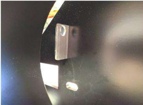
Figure 28: Air Temperature Sensor Installed onto Back Plate of Bumper
