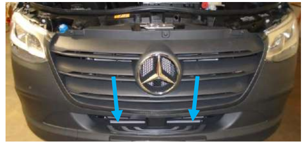
Figure 5: Plastic Cap Location
