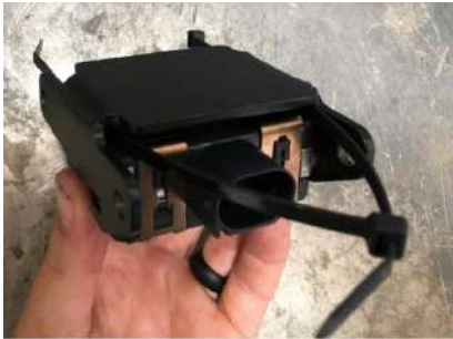
Figure 23: Feed a Zip Tie Between the Sensor and Sensor Carriage (Behind Sensor)
