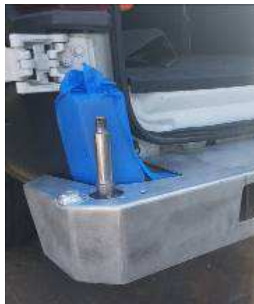
Figure 3. Tape applied to plastic corner pieces to prevent scratching. The swing arm has been removed and door is open to clearly show the location of the tape, although THIS IS NOT THE CONFIGURATION IN WHICH YOU SHOULD INSTALL YOUR ALUMINESS BUMPER.
