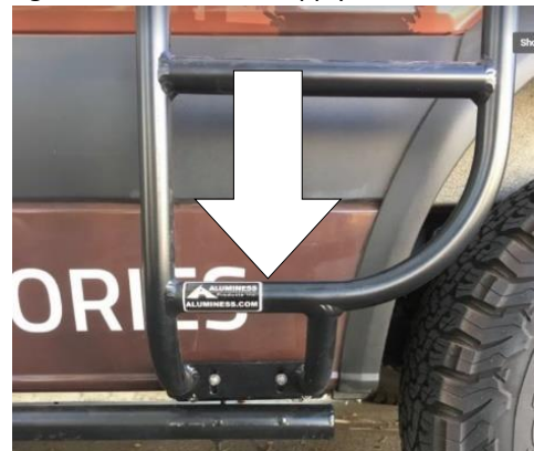
Figure 4: Lower Bracket Tightening Technique.
