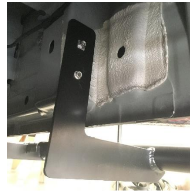
Figure 3: Rear Blade Secured into Position
