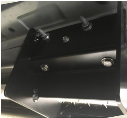
Figure 1: Hardware Installed Through Nerf Bar Brackets
