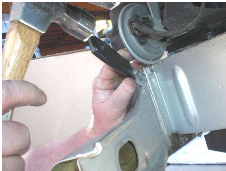
Figure 7: Releasing stock bumper with hammer and putty knife
