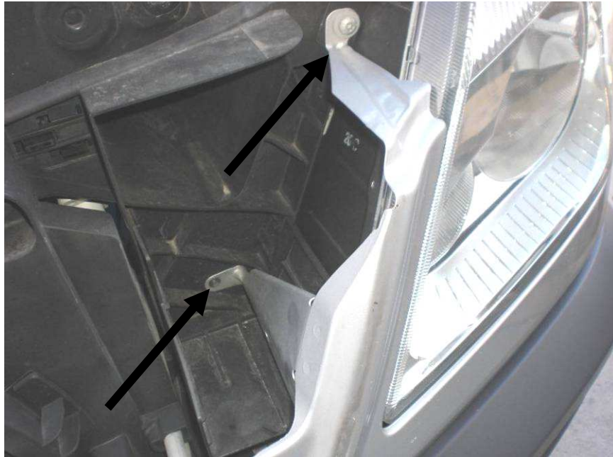
Figure 5: Headlight trim piece torx bolts
