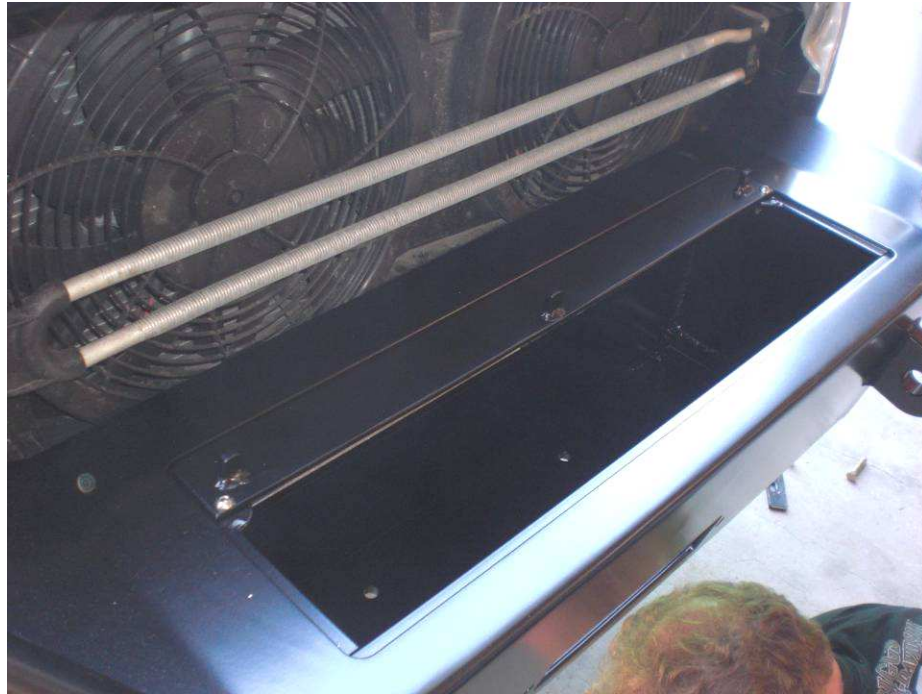
Figure 12: Bumper door, rear portion installed
