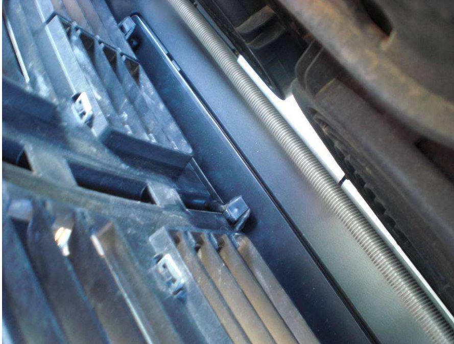
Figure 13: Stock grill installed on Aluminess door tabs
