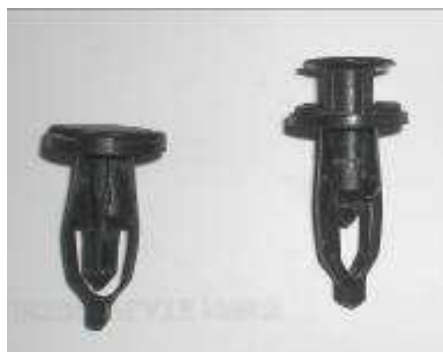
Figure 4: (Clockwise from top left) Plastic fastener location in fender well; Plastic fastener locations under leading edge of bumper; Plastic fastener closed (left) and open (right)
