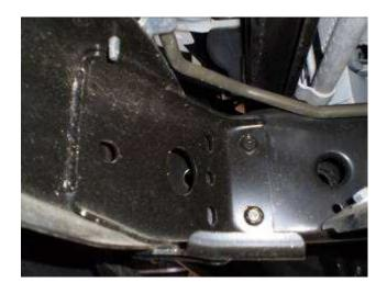
5. Once the Skid Plate is removed you should be able to unbolt the main bumper structure. There are 3 bolts on each frame rail that are accessed through the front of the bumper. You will see a 4th bolt on each side that does not actually hold the bumper on, but part of the inner bumper structure. You can remove this bolt as well if you would like.
