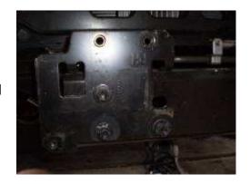
10. You are now left with a crossmember that needs to be removed. There are a couple of very large bolts that hold this crossmember on as well as a weld on the outer side of it. Remove the bolts so that the only thing holding the crossmember on is the weld.
