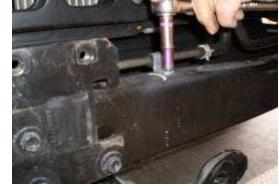
8. Take off the 2 bolts holding the cooler lines to the crossmember.
