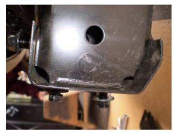
12. If you are unable to get the cutoff wheel along the entire weld then it may be necessary to break the ends loose with a hammer and chisel.
