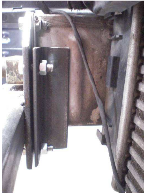
Figure 9: Attach the 2" X 1" angle brackets to the aftermarket bumper mounting plates (this is the passenger side)
