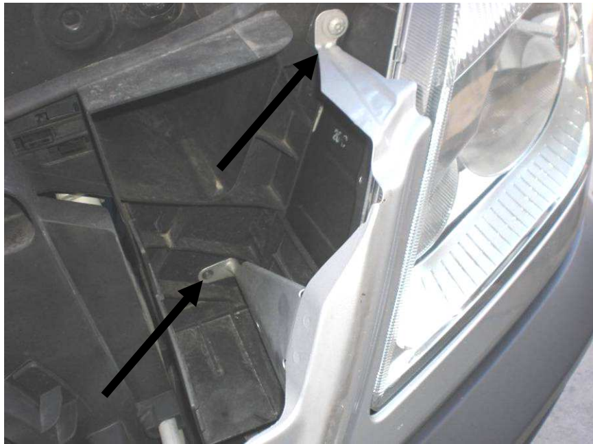
Figure 5: Headlight trim piece torx bolts
