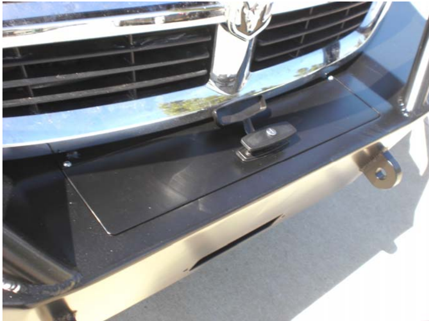
Figure 14: Bumper door installed
