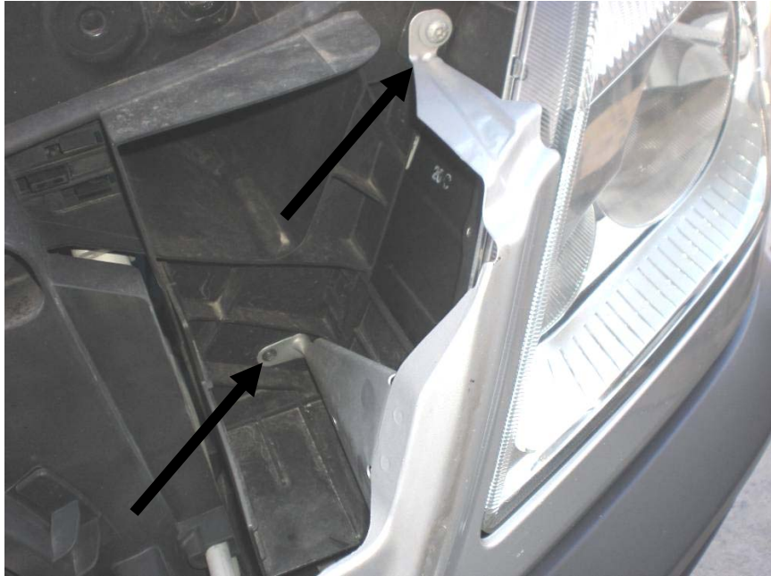
Figure 5: Headlight trim piece torx bolts
