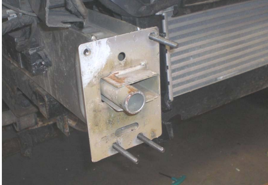
Figure 8: M8 bolts installed on passenger side frame horn
