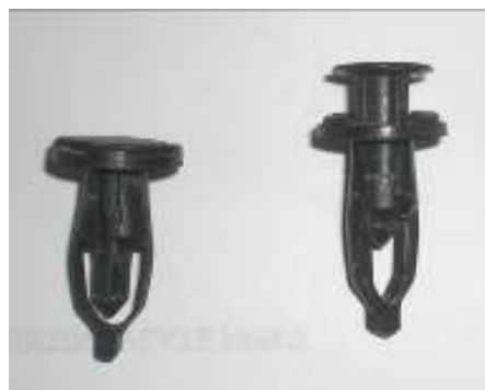
Figure 4: (Clockwise from top left) Plastic fastener location in fender well; Plastic fastener locations under leading edge of bumper; Plastic fastener closed (left) and open (right)
