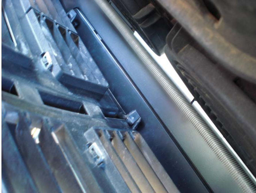
Figure 13: Stock grill installed on Aluminess door tabs
