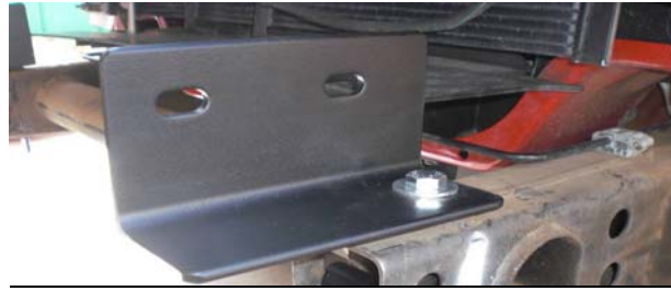
Figure 4: Installed bumper bracket
