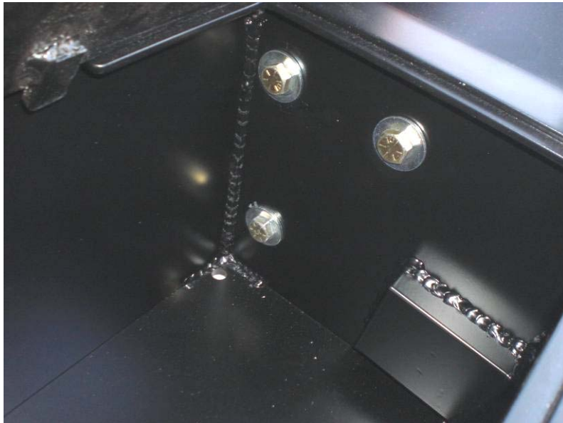
Figure 6: View of toolbox inside, showing correct orientation of mounting hardware
