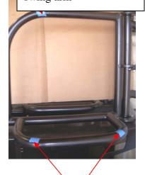
Location for bolts that are through bottom of box and swing arm
