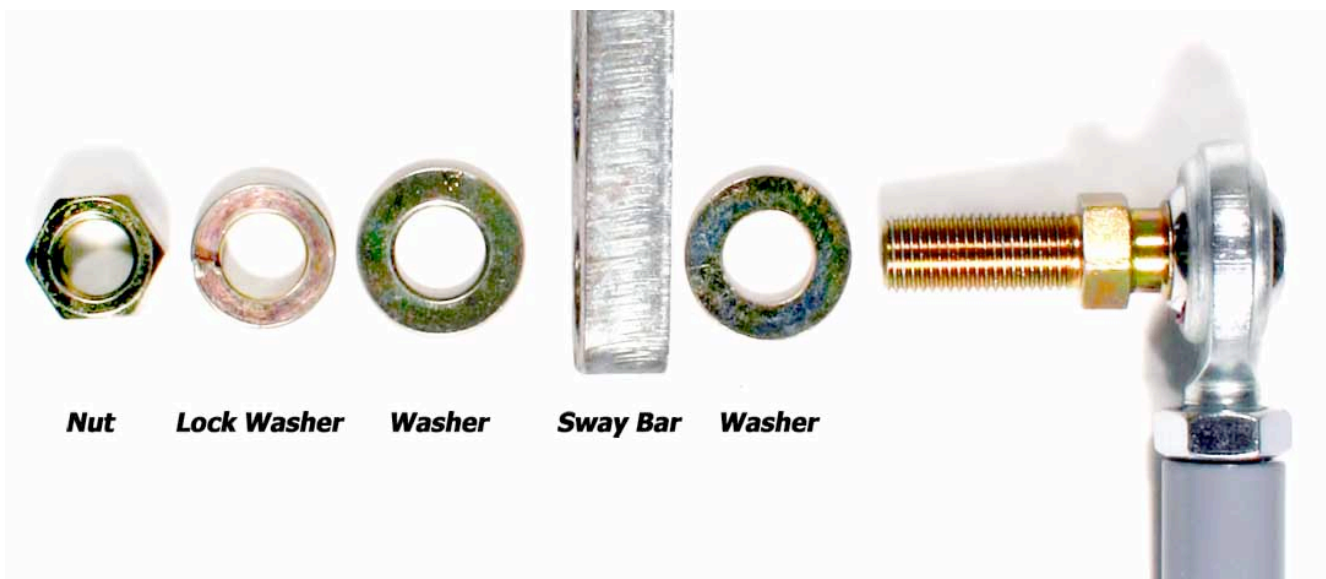
SHOWS SWAY BAR CONNECTION, AND PLACEMENT OF WASHERS
