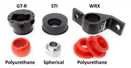
There are a few applications where a spherical bearing could be used, but it adds huge amounts of complexity to the part or sacrifices some amount of durability. For instance on the Nissan GT-R, we used a hard polyurethane instead of the bearing because we needed to be able to adapt our part to the OEM control arm. Same goes for the MINI Coopers as they have a strange hex shape that we adapt to, and it was easier to make this out of polyurethane.
