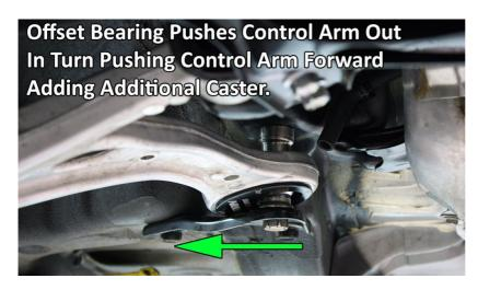
So why doesn't everyone get the offset bushing version of the PSRS? The only issue comes up when customers have really wide wheels and tires. Since we push the front wheels forward to get the extra castor, it pushes the wheels and tires closer to the fender liner. This mainly occurs on the 2008+ cars where 275 wide tires are a common upgrade. If that is an issue for you, then simply purchase the normal (zero offest) PSRS and you will have no tire rubbing or clearance issues at all.
