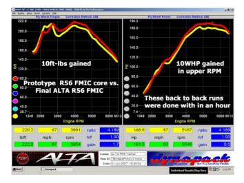
This test is with the prototype intercooler and final design ran back to back, and with-in minutes of each other. Just like we expected to see, more WHP at the upper RPMs. Not only is the overall WHP it gains very noticeable, but the ALTA FMIC looks really awesome on the car!
