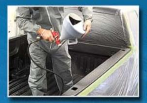
Al's Liner Air Texture Gun allows users to vary the texture and thickness of Al's Liner coating effortlessly. Al's only requires a 7 CFM air compressor with 25 to 55 PSI at the gun. Many textures can be achieved by adjusting the air pressure and amount of trigger pull. Includes locking trigger control for uniform coating. For best results, it is recommended to install an air regulator for better air pressure control. Gun includes: 1.5 gallon hopper and 6, 8, and 9.5 millimeter spray nozzles.
