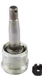
Due to precision tolerances please follow these steps. BEFORE installing, apply a small amount of grease, then rotate the stud back and forth ensuring movement is free. If over greased you will need to remove the grease fitting to release pressure.
