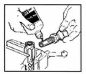
Lubricate nipple and threads LIBERALLY. Use heavy oil or hose assembly lube.
