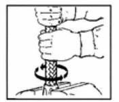
Put socket in vise and rotate hose counterclockwise into socket until it bottoms, then back off 1/4 turn. When assembling long lengths of hose put the hose in vise just tight enough to prevent turning and turn socket into the hose counterclockwise until it bottoms.
