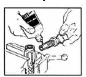
Lubricate nipple and threads LIBERALLY. Use heavy oil or hose assembly lube.
