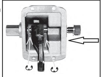
Step 5. Center the slip collar in the axle housing locking both axle halves together. Install the new cover and gasket onto the axle aligning the fork into the slip collar.
