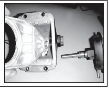
Note: If your vehicle was equipped with a vent tube in the original housing it will need to be reused in the new housing. If your vehicle did not have a vent tube then the supplied plug will need to be installed using thread sealant.
