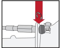
Step 11. Locate the vacuum switches on the passenger's side firewall.
