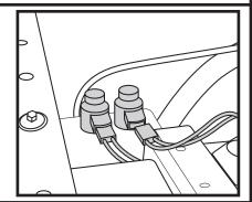
Engaged- Place the transfer case into four wheel drive. Press and hold the red push button on the control cable and pull the cable outward. The vehicle may have to roll slightly for the coupler to fully engage. Once the cable lock has fully engaged adjust the hold/release knob clockwise to secure the cable.
