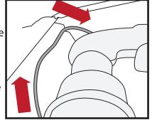
Step 6. Thread the supplied jam nut on to the end of the cable as far as you can. Apply RTV silicon sealant to the threads on the end of the cable. Install the supplied brass housing on to the cable and tighten down. Do not over tighten. Thread the brass fitting on by hand until it bottoms out on the cable. If the fitting is over tightened, the knob will begin to extend and you will need to back off the brass housing. Tighten the jam nut against the brass housing to secure the housing.
