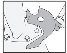
Step 4. Remove vacuum diaphragm by using a rubber mallet to tap on brass part of the diaphragm. If the vacuum diaphragm cannot be removed by hand use a hack saw (fine tooth) to remove plastic diaphragm. Note: You will be cutting through plastic, brass and steel. Cut directly next to the aluminum mount on the passenger's side of the mount.
