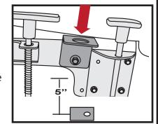
Step 2. Remove the jam nut and washer from the handle end of the cable. Start cable through the dash bracket. Place nut and washer over the end of the cable and continue the cable through the hole drilled in the firewall. Fasten cable loosely to the dash bracket with the jam nut and washer. Cut grommet on one side to form "C" and install grommet in the firewall to protect the cable from the sharp metal. Note: may want to put silicone lubricant on grommet for easier
