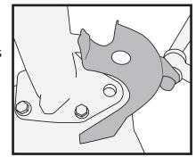
Step 8. Clean the factory mounting surface using an emery cloth.
