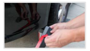
Firmly press the tape attached to the lip against the lower portion of the bumper.
