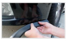
Around curved parts of the bumper, cut a "V" in the lip to allow for a clean bend around the bumper.
