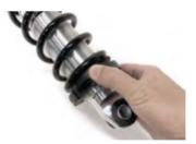
Step 3. With anti-seize applied on your spring retainer threads, set screw installed (hand tight at this point); thread the retainer onto the coilover shock body.
