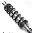
Step 6. Retainer should be tight on the shock body with zero movement or play once installed. Your spring and spring retainer installation is now complete.
