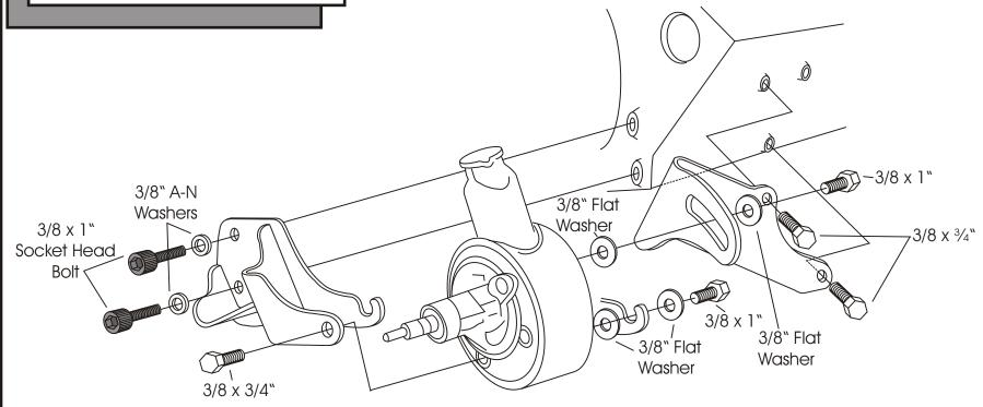
NOTE: If your pump has a stud at the lower rear pivot point, it must be removed and the 1" bolt and 3/8" flat washers used..
