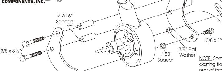
NOTE: Some early blocks may have casting flash that will interfere with the rear of bracket. This is easily removed with a small grinding stone or hand file.
