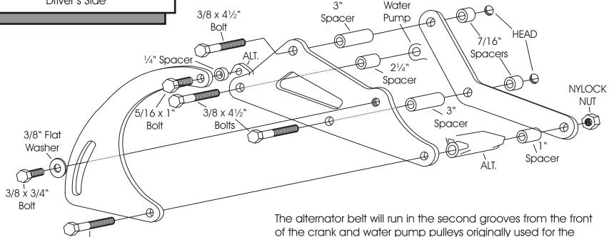
It can be used with single groove crank and water pump pulleys by using a double groove alternator pulley and running the belt in the outer groove.
