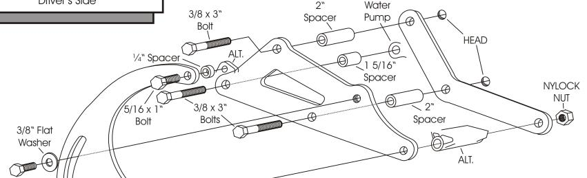
As with any mount system, assemble all of the brackets to engine BEFORE TIGHTENING THE BOLTS.
