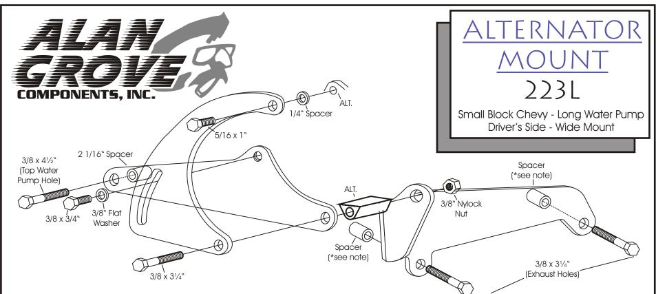
\*NOTE: <u>Exhaust Spacers</u> - with HEADERS - use the  $2\frac{1}{4}$  long x 5/8" O.D. Spacers. With RAMS HORN MANIFOLDS use the  $\frac{1}{4}$ " long x 3/4" O.D. Spacer at rear hole of bracket and a 1 1/16" long x 3/4" O.D. spacer at front hole of bracket. With the later DROP-TYPE MANIFOLDS use the 1 1/16" long x 3/4" O.D. Spacers at both bracket holes. As with any mount system, assemble all of the brackets to engine BEFORE tightening the bolts.
