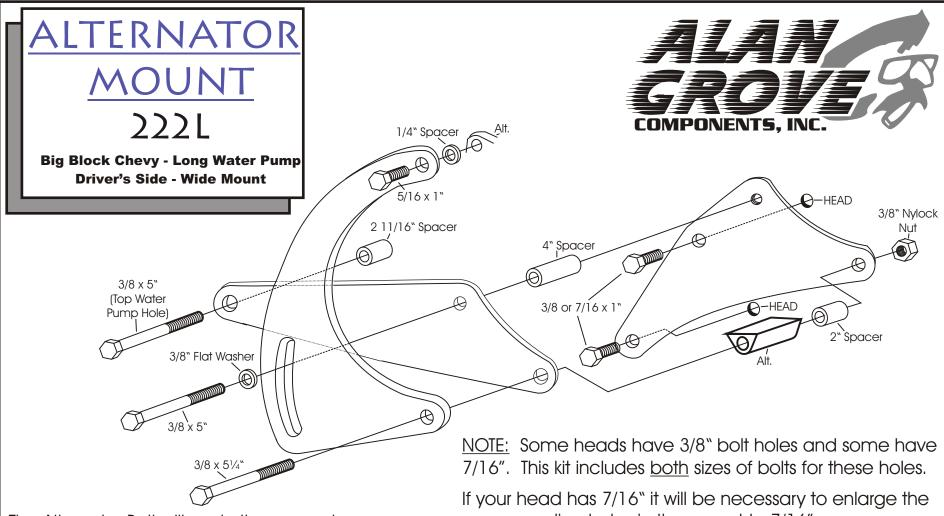
The Alternator Belt will run in the second grooves from the front of the crank and water pump pulleys originally used for the factory compressor. It is designed to be used with our 122R Passenger Side Compressor Bracket.
