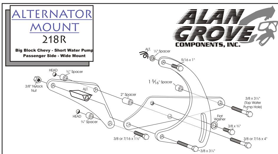
(We use a belt length of 58-59" with this mount on installations in our shop. However; this can vary with the diameter of your pulleys.)
