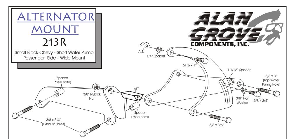
We use a belt length of 57-58" with this mount on installations in our shop. However; this can vary with the diameter of your pulleys.
