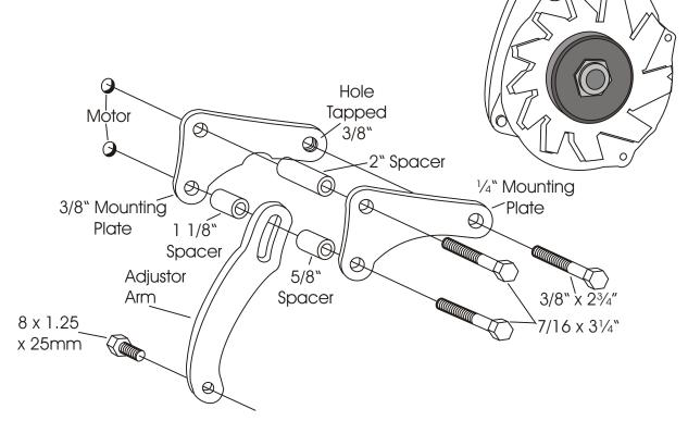
This bracket is designed to be used with the small CS 130 G.M. Alternators with the threaded mounting ear in the 2 o' clock position.
