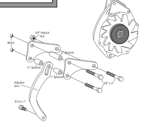
(We use a belt length of  $42\frac{1}{2}$  to  $43\frac{1}{2}$ " with this mount on installations in our shop. However; this can vary with the diameter of your pulleys.)
