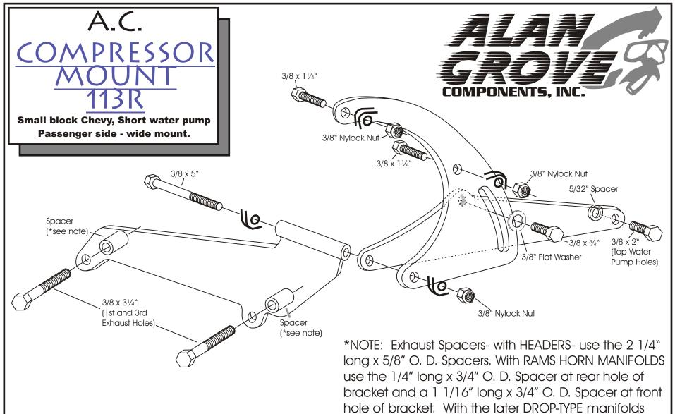
We use a belt length of 60-61" with this mount on installations in our shop. However; this can vary with the diameter of your pulleys.
