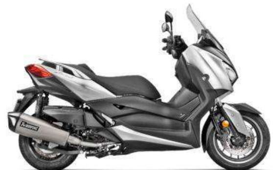
Yamaha X-MAX 400 + 1.7 HP/6,050 rpm - 4.8 kg (-45.7%)
