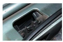
5. If the hood is not aligned properly, adjust accordingly and tighten bolts at the hinges.
