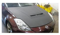
3. Tighten bolts to just enough torque to hold the hood in place, but lose enough to be adjusted by a tug.
