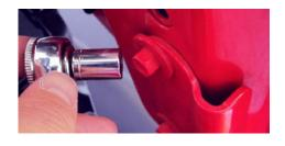
6. Re-install hood latch and adjust for fitment. (If the hood is latched but not fully close, the latch might need to be adjusted shorter. If the hood does not latch down, the latch might need to be adjusted longer.
