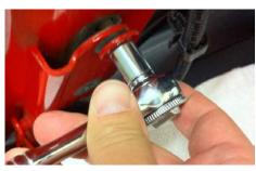
4. Remove hood latch and check alignment.
