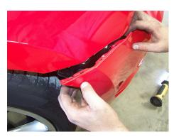
8. When you are satisfied with the fitment, mark the holes needed for the installation and cut or drill accordingly. (Be very precise in making hole, as this will determine the accuracy of the fitment to the other panels of the vehicle.)
