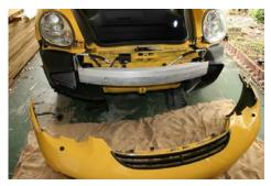
5. Some installation will require removal or repositioning of factory components, like impact absorbers, reinforcement bars, horns or fog lights. If any component is interfering with the installation, remove these components and proceed with test fitting the bumper. (Make sure to reinstall all vital components back in its place or new location. Some products are meant for show and off-road purposes only. Removal of any factory safety components are at your own risk.)
