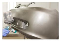
10. After the paint has dried, you are ready to install the bumper on to the vehicle. After part installation onto vehicle, you may wet sand the clear coat then buff to achieve the shine.
