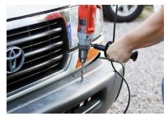
7. With the bumper mocked up in place, make sure it lines up properly with rest of the panels and lights of the vehicle. (Some areas of the bumper are purposely made with extra material to lower the risk of damage during transit. Some bumpers might need to be shaved or filed down in some areas to insure a good fitment.)
