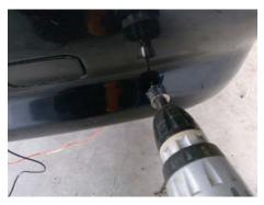
9. After holes have been drilled, your part is now ready to be prep for paint. Because of the characteristic of FRP composites, you would need to block (sand and fill, etc.) the whole bumper to ensure smooth and even application of paint.
