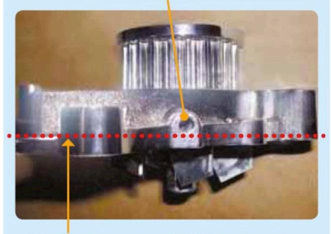
Submerge the water pump body below the red line
