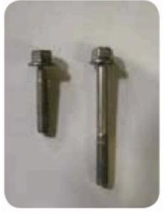
Torque Long bolt (A) 26N\*m Short bolt (B) 21N\*m
