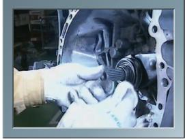
Use the clutch alignment tool to locate the clutch disc with the input bearing while tightening the clutch cover bolts. Tighten bolts with torque wrench in a diagonal (star) pattern.
