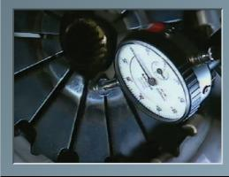
Align the input shaft correctly with the clutch disc.
