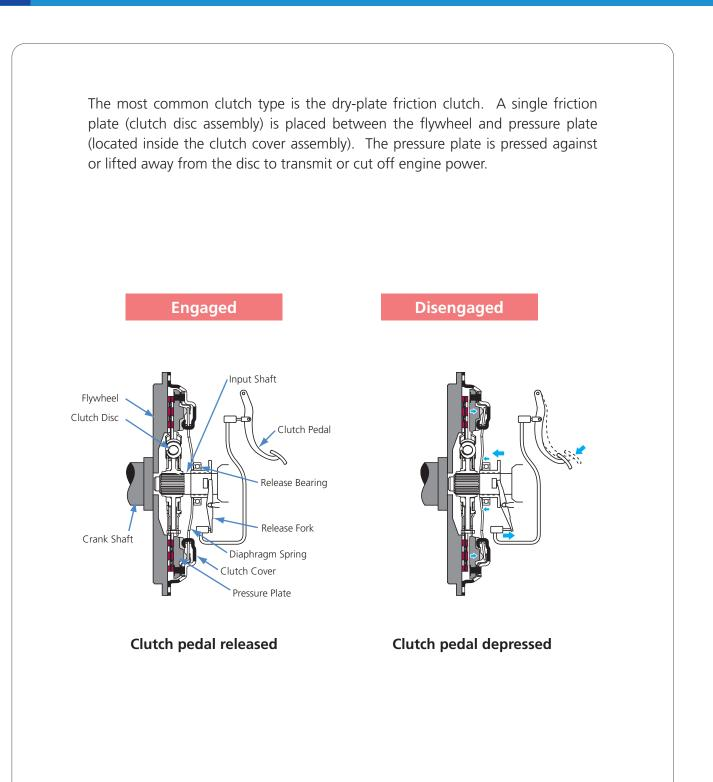
The basic components of a clutch system includes the clutch cover assembly (pressure plate, diaphragm spring, cover, etc.), clutch disc assembly, flywheel, release bearing, and release fork. The clutch disc is located between the flywheel and pressure plates and is connected to the transmission gears by the main drive shaft (input shaft).
