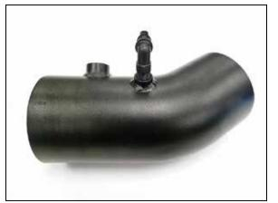
15. Install the provided 90° vent fitting into the AIRAID<sup>®</sup> intake tube as shown.
