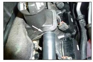
4. Disconnect the crank case vent hose from the valve cover.
