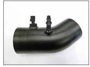
17. Install the inlet air temperature sensor into the AIRAID<sup>®</sup> intake tube as shown.
