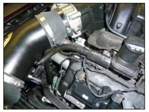
21. Install the assembled vent hose onto the fitting installed in the AIRAID<sup>®</sup> intake tube and then attach the open end to the valve cover port.
