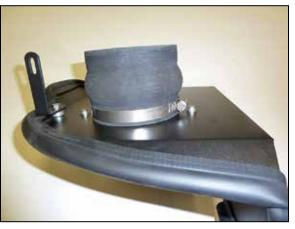
12. Install the provided hump hose (08418) onto the filter adapter and secure with the provided hose clamp.
