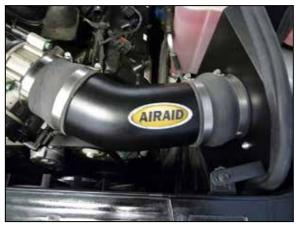
18. Install the AIRAID<sup>®</sup> intake tube into the silicone hump hose and then into the into the silicone step hose at the throttle body. Align the intake tube and heat shield for proper fit and then secure the intake tube with the provided hose clamps and the heat shield bracket with the factory air box retaining bolt removed in an earlier step.
