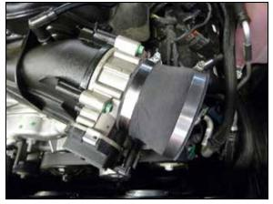
14. Install the step hose (08050) onto the throttle body and secure with the provided hose clamp.
