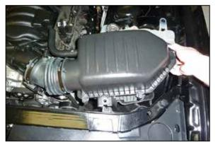
7. Lift up and remove the complete intake track from the vehicle.
