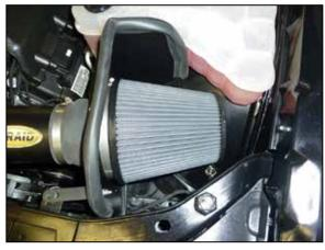
24. Install the AIRAID<sup>®</sup> air filter and secure with the provided hose clamp.
