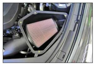
11. Install the AIRAID® air filter onto the intake tube and secure with the provided hose clamp.
