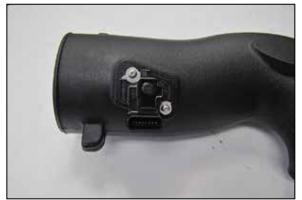
6. Remove the mass air sensor from the factory air filter housing and install it into the AIRAID® intake tube using the provided hardware.
