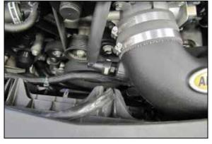
10. Connect the vent line to the quick disconnect fitting installed into the AIRAID® intake tube.
