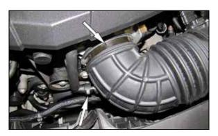
3. Disconnect the crank case vent line and loosen the hose clamp that secures the intake tube to the throttle body. Remove the complete intake system from the vehicle.
