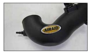
7. Install the provided quick disconnect fitting into the AIRAID® intake tube and then apply the provided decal onto the intake tube.
