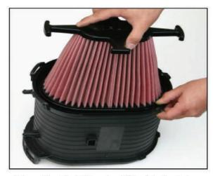
4. Insert the Airaid Premium Filter into the factory housing. The filter must be fully inserted into the bottom of the housing. Install the factory filter housing with the Airaid Premium Filter into the vehicle in the reverse order. Double check your work to insure that all connections are tight there are no foreign objects in the intake system.
