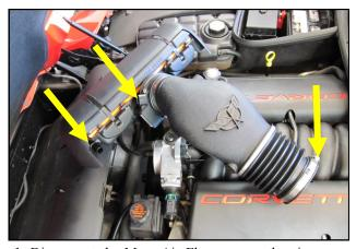
**1.** Disconnect the Mass Air Flow sensor, the air pump breather line and loosen the hose clamp on the throttle body. Remove the entire intake as an assembly and set it aside.
