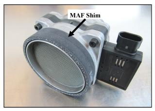
**4.** On 1997-2000 models the MAF shim will need to be installed for proper fit.
