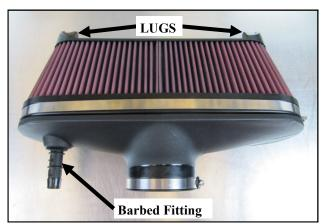
**3.** Create the Filter Assembly as shown using the supplied Grommet, Barbed Fitting and Hose Clamps. Refer to the Exploded Diagram for assembly detail. Note the location of the Filter location lugs and their position relative to the Barbed Fitting. Maximum Hose Clamp torque is to be no greater than 20 LB/IN.
